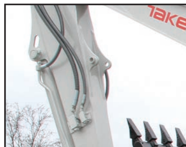
Auxiliary Hydraulic Lines
